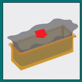
Insert the liner. This is available from C&B or you can use heavy duty plastic sheeting. Make sure you do not purchase a porous type. Push the liner right into the edges.
