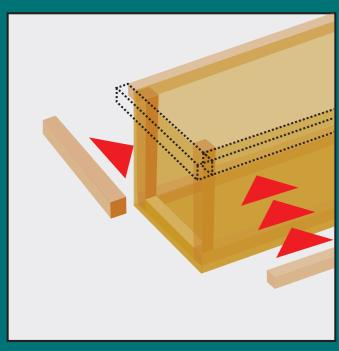
Fit edge reinforcing timber to the outside edge around the top. Do not skip this part as the weight of water will otherwise distort the OSB. The edge timber also provides a convenient place to staple your liner.
