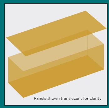
The panels can be lightly nailed, glued or screwed together to form the basic box. Make sure you have a lid to stop pets or children gaining access. The box now needs reinforcing with the 40mm timber at its joins and edges.
