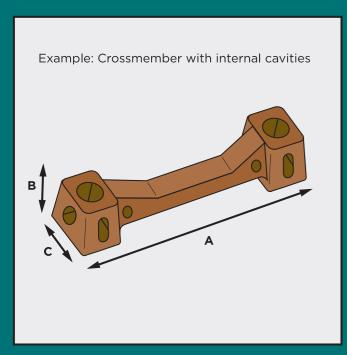
Measure the overall size of the biggest item you want to IReOx and add about 20% in each direction. It is most economical to take into account the dimensions of the sheet material you are using, usually around 2400 x 1200mm (8x4')
