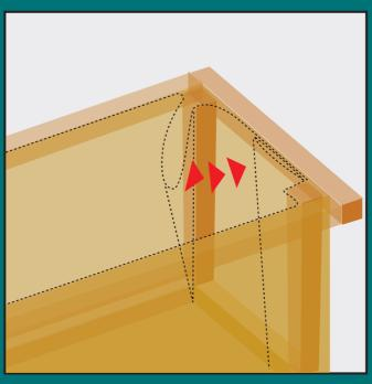
Fold the excess in at the corners as shown. Make sure that no edge is going to be below the level of the IReOx. staple, tape or tack the liner to the top edge reinforcer.
