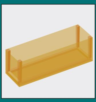
Cut the timber to fit inside the corners and screw through the OSB into the timber. Make sure no fasteners extend into the box as they may pierce
