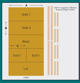
The most economical material we've found that is sufficiently moisture resistant to be used outdoors is 'OSB3' (not 1 or 2). Good timber yards will have a cutting service that is cheap or even free. Making use of it makes your material easier to transport and quicker to assemble.
